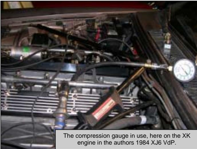
The compression gauge in use, here on the XK engine in the authors 1984 XJ6 VdP.
