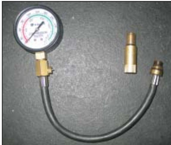
Two types of compression gauges. The preferable type is that above, which threads into the spark plug hole for a positive seal. Note the adapter which provides additional thread sizes to allow use with most vehicles. The type of gauge below requires careful alignment and steady holding pressure to ensure the rubber plug seals properly.
