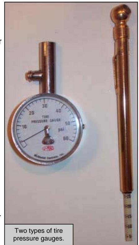
Two types of tire pressure gauges.
