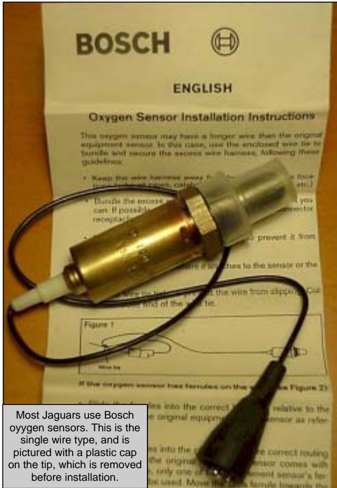
Most Jaguars use Bosch oxygen sensors. This is the single wire type, and is pictured with a plastic cap on the tip, which is removed before installation.
