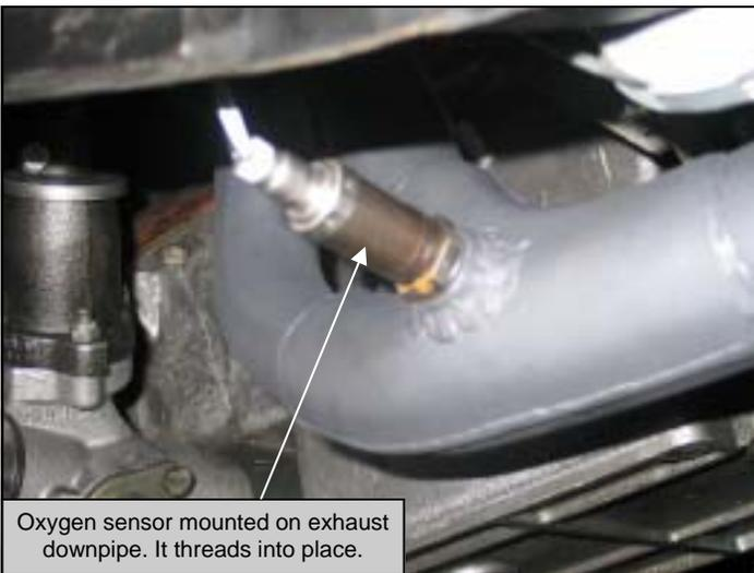
Oxygen sensor mounted on exhaust downpipe. It threads into place.
