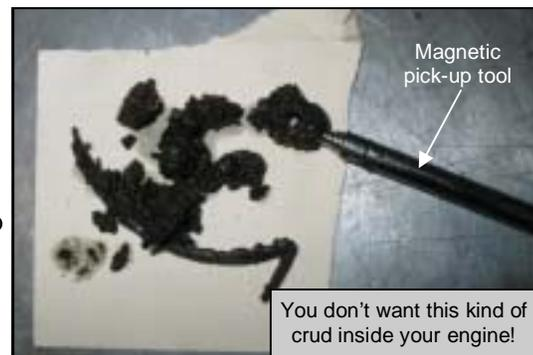
I had to repeat the flush and suction process a few times, and I even tried pouring water through a funnel directly into the stud holes from above, but eventually I was rewarded with clean flushing water and crud free holes, ready to accept the new studs. What fun! Now it's onto the next challenge!
