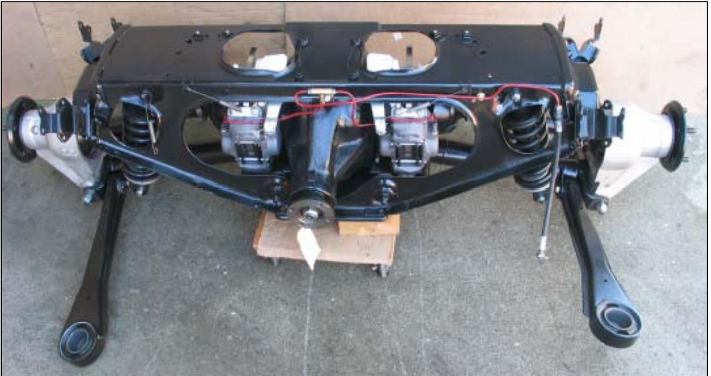
After World War II, Jaguar chassis engineer Bob Knight did some investigating into independent rear suspension systems (IRS) with the intent to fit one in upcoming models. A system, originally patented by Georges Roesch of Clement Talbot Ltd, was generally accepted by Sir William Lyons and the rest of Jaguar management, but was then set aside. Ten years later, in the 1950s, Jaguar considered their existing chassis rather outdated, and revisions were considered vital for the new series of cars.
