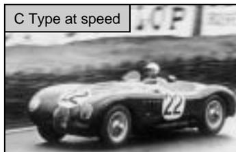
hour. The XK120C, or C-type, was designed for competition, with a 210 hp engine, all aluminum body, independent front suspension, and torsion bar rear suspension. The body was attached in three sections
