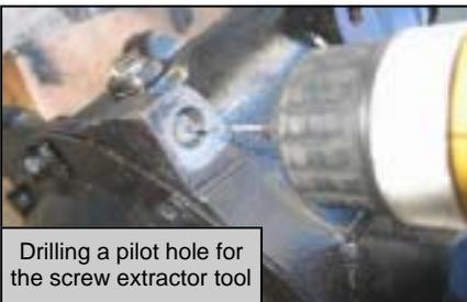
I then applied a little fastener-release lubricant to the hole. The one I use is called Moovit - there are others such as Kroil, Busty, and even Rust Check can help. I do
