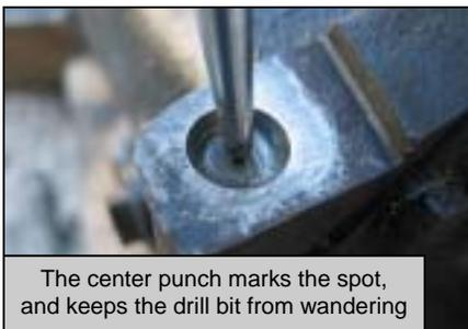
I decided to try my luck with a screw extractor, so I hoisted the heavy differential onto my workbench, and used a punch to make a dent in the center of the broken bolt. This keeps the drill bit from wandering. Using a drill bit of a size appropriate for the diameter of the extractor tool, I drilled a pilot hole approximately 1/4" deep into the broken bolt. It's important to not drill through the end or sides of the bolt - the idea is to get it out with no evidence that there was ever a problem.
